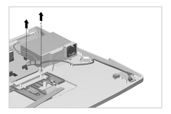
Figure 7-29. Disconnecting the IrDA Board
